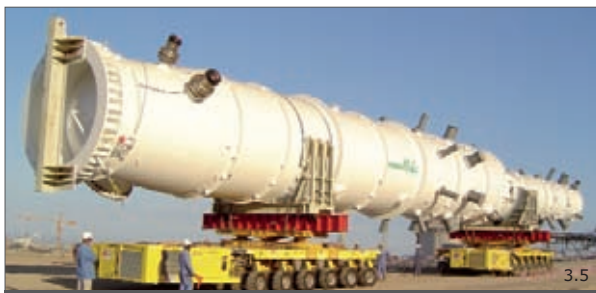
SPMTs in loose coupling mode. Vehicles are connected with only one data line and controlled with only one operating panel.
